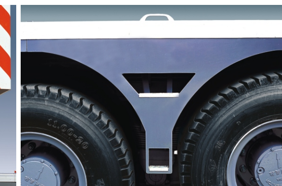
● 方便的上车楼梯 ● Convenient stairs for getting on the crane
