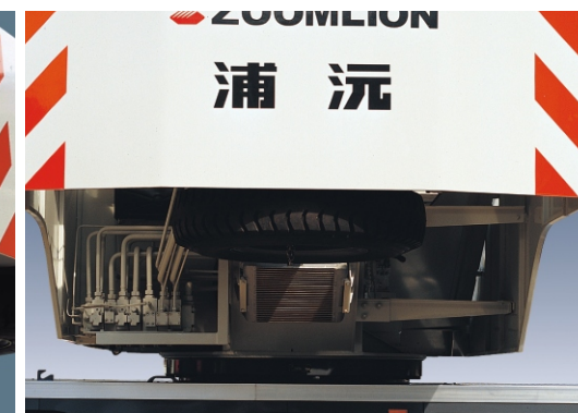
● 收放自如的备胎升降机构 ● Spare tyre mechanism freely extending & retracting
