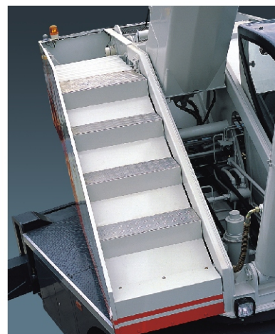
● 方便的转台楼梯 ● Convenient stairs of swing table
